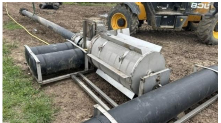
Figure 3, Tom's pontoon filter ready for installation in November 2023.
