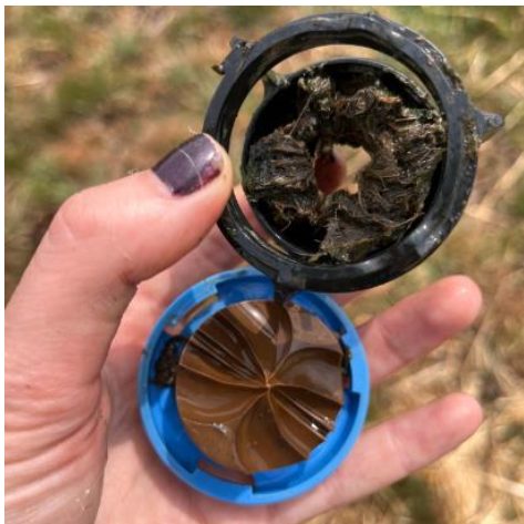
Figure 2, One of the nozzles on Tom's pivot showing blockage by effluent particles.
