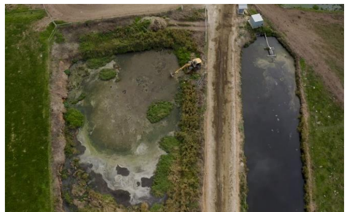
Figure 1, Tom's two pond effluent system.
