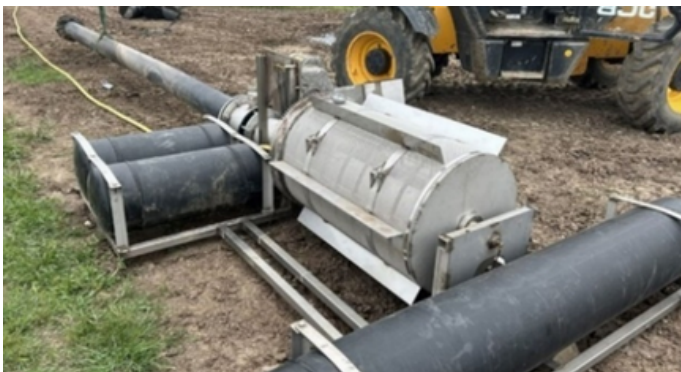
Pontoon filter ready for installation, at a cost of $28,000
