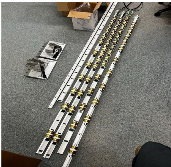
1.9m soil moisture probes pre-installation at the demonstration site
